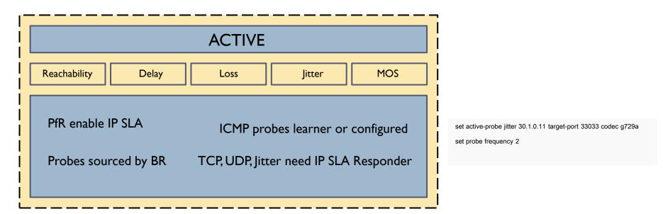
In this mode, IP SLAs probes are generated by the border routers through the current exits and transmitted at the configured probe frequency value. Probes are only generated through alternate paths (exits) in the event the current path is out-of-policy.
