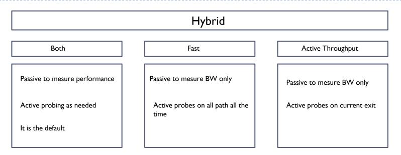
Mode monitor both is the default value and combines the capabilities of passive and active monitoring. Up to five IP addresses are actively probed for each destination prefix network learned through passive monitoring. By default, an IP SLA ICMP ECHO probe is automatically generated for the learned IP addresses.
